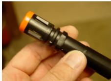
And fit it so you can mount it on the rear of the airsoft receiver. You will want to use a dremel or round file, and contour the receiver to this barrel tip can sit even. Mix up some plastic welder or epoxy and
