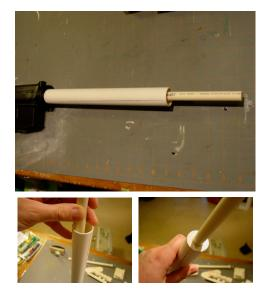
parts. And then insert the barrel. Be sure to seat the barrel al the way down! Next we started trimming the barrel adaptor plug. This should be tight so trim and fit as you go. Clean up the front sight and barrel band.
