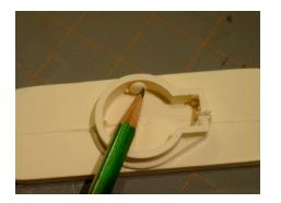
Start with the parts laid out on a table, and sand or trim any flashing or excess materials off each part. The stock greebly, top pipe adaptor, butt plate and scope front all have sprues that need to be cut off and sanded. Also note the surface finish is rough, and you might
